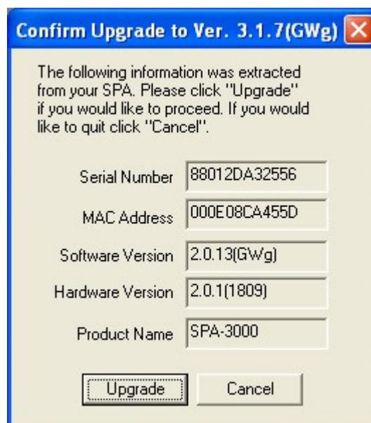
Click on the Upgrade button to begin the upgrade procedure. The upgrade itself should only take a minute or so. Whatever you do don't turn the power of during this operation.
